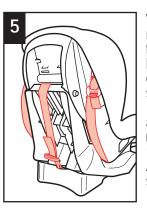
When LATCH is not being used, fasten LATCH hooks on side of child restraint as shown. Hook top anchorage strap to recline foot (see "Adjusting the Top Anchorage Strap" section).
